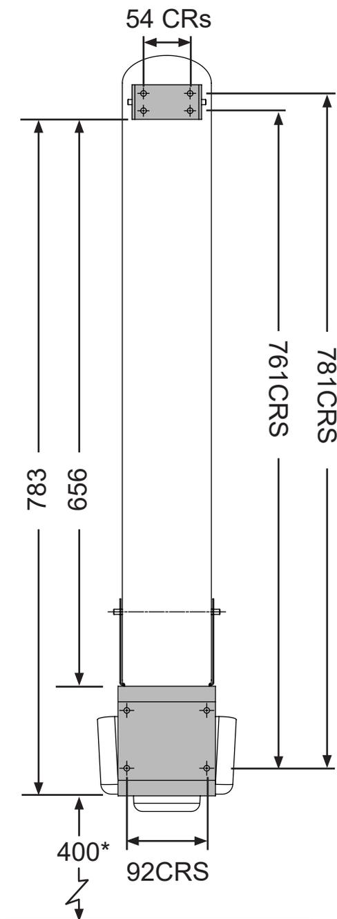
\* LE SUPPORT DU PLATEAU D'ÉGOUTTEMENT DOIT ÊTRE INSTALLÉ À 400mm AU-DESSUS DU SOL
